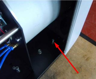
6) Remove the 4 screws holding the front cover to the base, 2 each side
