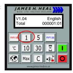
Pressing button number 1 again turns the reversing mode on/off . Reversing mode is on when  $\uparrow\downarrow$  is displayed at the top left of the screen.
