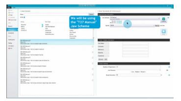
Select the "T27 Manual" Jaw Scheme Check that the T27 Grips are physically connected to Titan and click the Confirm button
