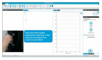
Place the Hook Holder attachment centrally in the top jaws and adjust the screw to just hold it
