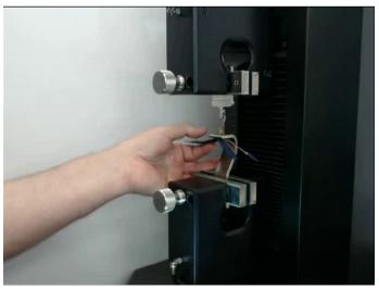
Insert the zip puller, from below, into the Puller Fixture
