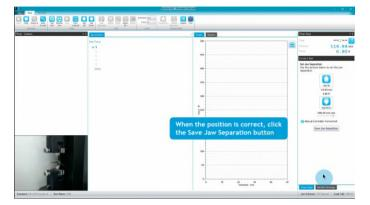
When the position is correct, click the Save Jaw Separation button
