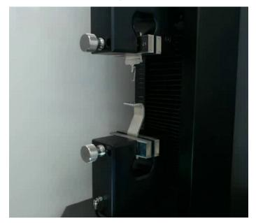
Finally, insert Hook (of suitable size for the puller being tested) into the Hook Holder
