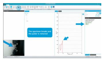
The specimen breaks and the puller is removed from the slider.
