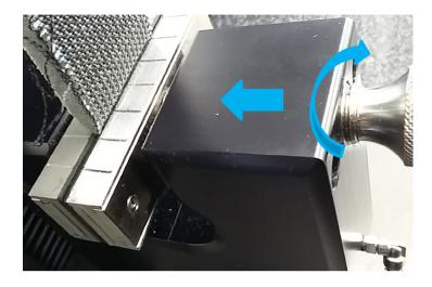
Then proceed as usual to close the top and bottom jaws pneumatically using the Titan Button or the Foot Switch.
