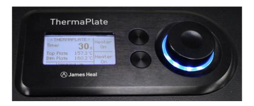
Set the timer to the required test duration by turning the selector button to <TIMER>. Select by pressing and then rotate to desired time. Press again to select and it will return to the home screen.
