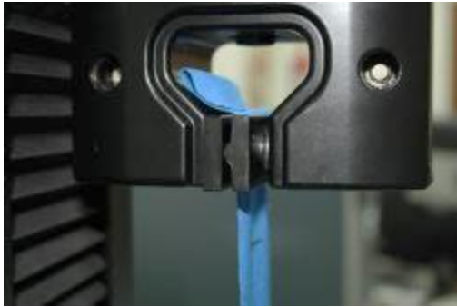
Above: Line Contact jaw faces
