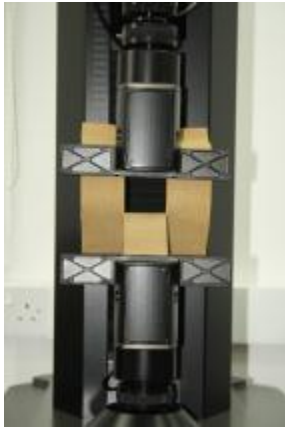
Tongue tear (or double-rip) tear specimen ISO 13937-4
