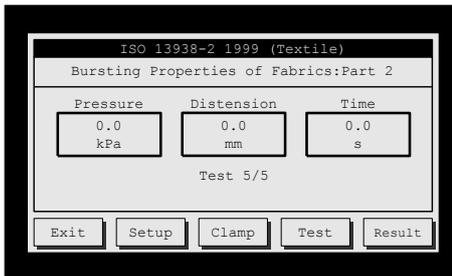
Place your specimen under the dome and make sure it is perfectly flat. Press the **Clamp** key and the clamp will be lowered.
