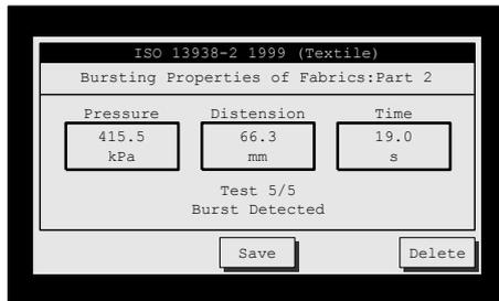
TruBurst<sup>3</sup> will automatically stop if it detects a burst and will display the final test result.
