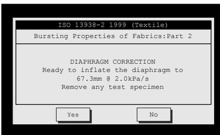
Once required number of tests have been fulfilled it will take you to the Diaphragm Correction screen, if you require diaphragm correction press **Yes** if you do not press **No**.
