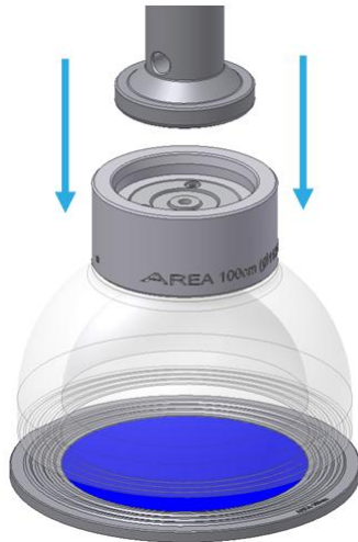
Figure 7: Removing the Test Dome
