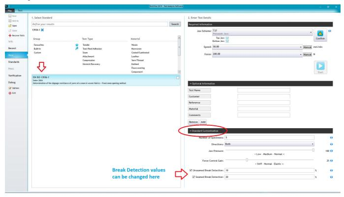
To change Break Detection value during the test (between specimens), go to File > Info > Edit:
