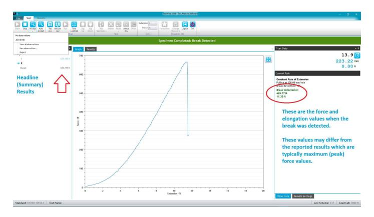
When TestWise detects a break it is saying that the break was detected when the force was 665.77 N and 11.38 % elongation, like co-ordinates on the force/extension curve.
