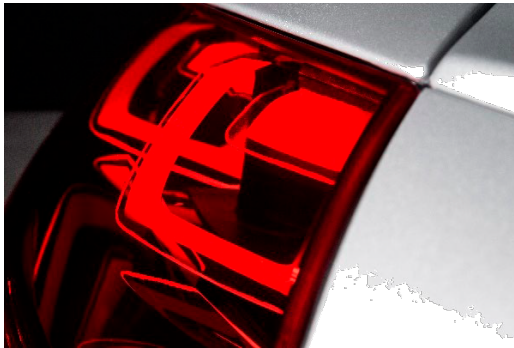
Figure 8: Principle illustration, flexible OLED following curvature of car shape and lamp curvature of AUDI TT
