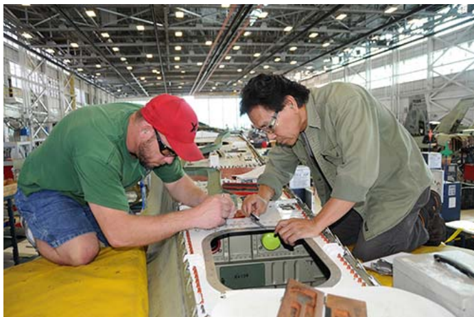
Lonnie Conditt, left, and Narom Orr, right, both machinists at Fleet Readiness Center Southeast in Jacksonville, Fla., measure holes to ensure alignment of an F/A-18 Hornet part on the production line. (Photo by Victor Pitts)
