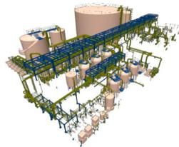
**Figure 1: An example of tridimensional model created by CAD 3D tools that could be used at BIM**
