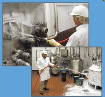
Foam cleaning is recognized as an effective method for removing organic and inorganic soils from all types of surfaces. It is used for cleaning throughout the food processing, dairy, transportation, industrial and agricultural industries.
