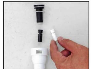
A unit can be changed from a 3.8 LPM unit to a 15.2 LPM unit with a switch of the venturi.
