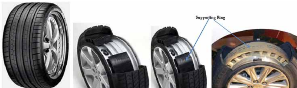
Fig.4: Supporting Ring System
