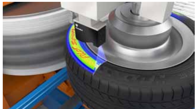
Gocator 2530 high speed 3D blue laser profiler scanning a tyre sidewall
