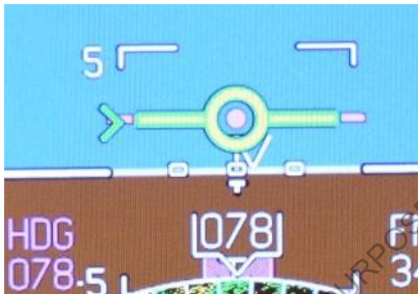
Figure 9-10-20 Non Conformal FPS
