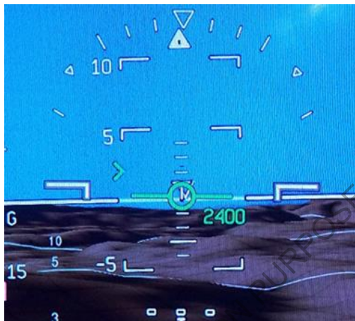
Figure 9-10 24 Acceleration Chevron above FPS: Aircraft accelerates (aircraft is in level flight in this example)
