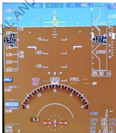
Figure 9-10-19 FPS with Compressed Pitch Scale
