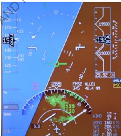
Figure 9-10-13 Excessive Bank Angle
