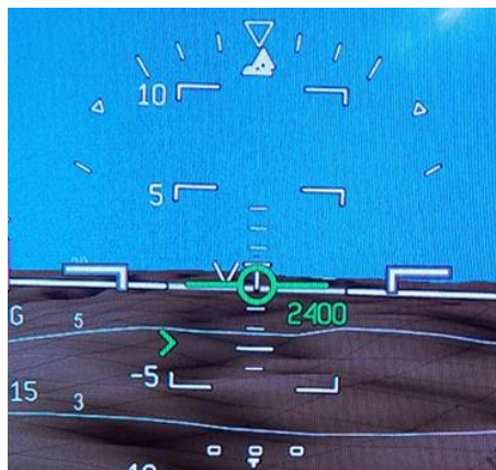
Figure 9-10-26 Acceleration Chevron below FPS: Aircraft decelerates (aircraft is in level flight in this example)
