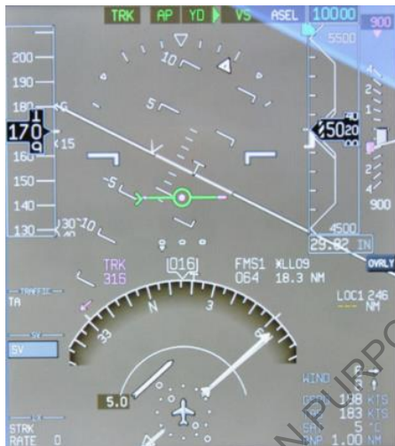
Figure 9-10-12 Synthetic Blue Display
