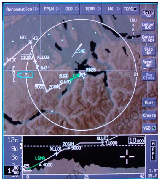
Figure 7-38-1 Vertical Situation Display
