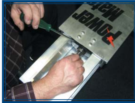
Pic L - B: Hand tighten the Ballnut Locknut
