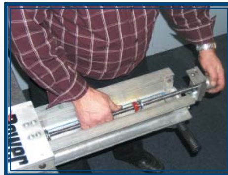
Pic I - N: Turn stairclimber drive screw so the ballnut is positioned halfway along the drive screw.
