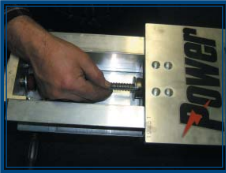
Pic L - A: Loosen the two set screws
