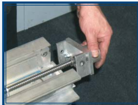
Pic M - F: Fasten bearing retainer to inner frame.
