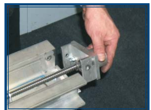
Pic I - O: Grip the drive screw and rotate to engage the coupling with the spline on the stairclimber motor.
