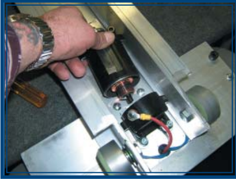
Pic I - G: Gently grasp top and middle of motor
