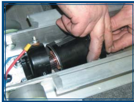
Pic I - K: Put motor body on a slight angle and join together.
