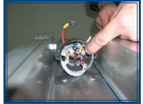
Pic I - I: Place the new motor brush into the casing
