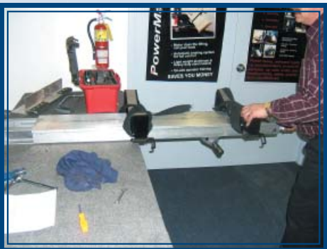
Pic I - D: Slide off the outer frame from the inner frame
