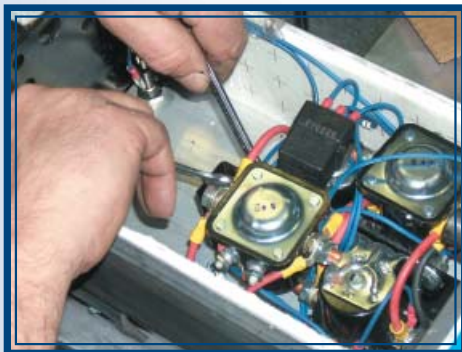
Pic F - D: Loosen only and remove relay
