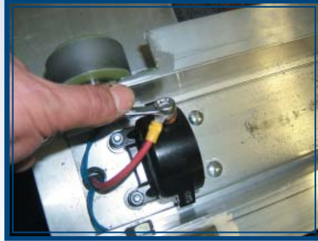
Pic I - H: Loosen up the bolt on the casing that is still attached to the frame.
