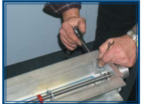
Pic M - C: Remove the tow bolts and nuts fastening the bearing retainer.
