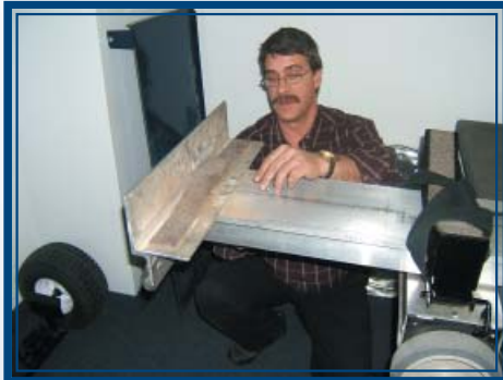
Pic M - B: Remove four nuts retaining the toeplate to the outer frame.
