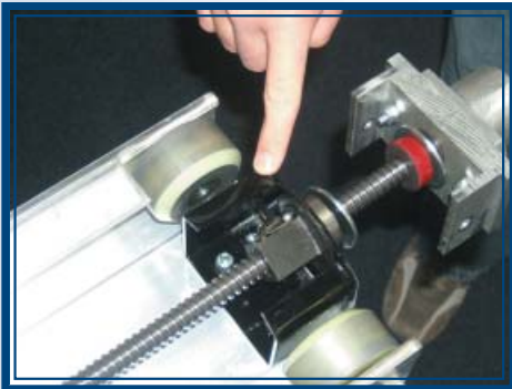
Pic M - D: Remove the four nuts on Ballnut Bracket
