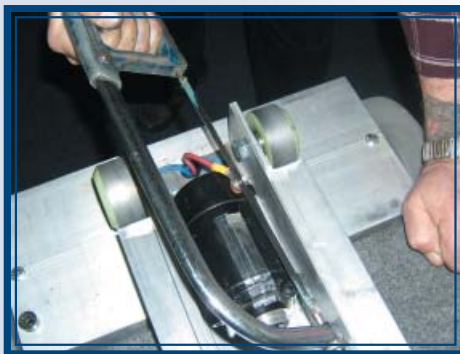
Pic I - M: Take a hack saw and cut off excess bolt even with the nut on the motor brush
