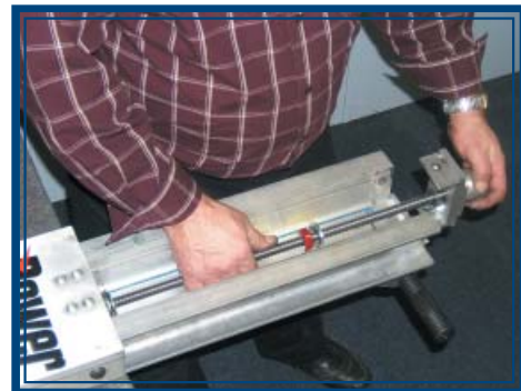
Pic M - E: Slide outer frame over the inner frame.
