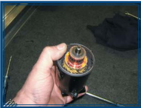
Pic I - J: Check the motor spline and ensure there are still three washers on the spline
