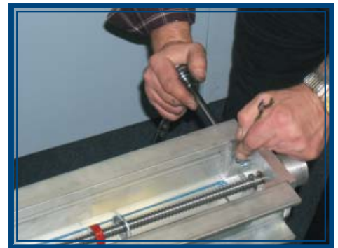
Pic I - C: Remove teh two bolts and nuts fastening the bearing retainer
