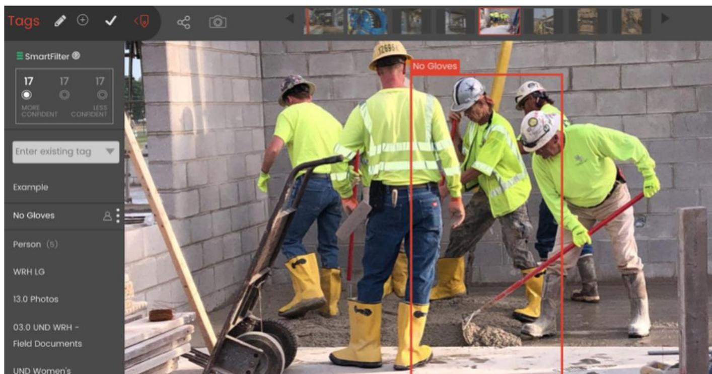
Smartvid.io's artificial intelligence system can detect when construction workers are not wearing gloves or other protective gear. SMARTVID.IO
