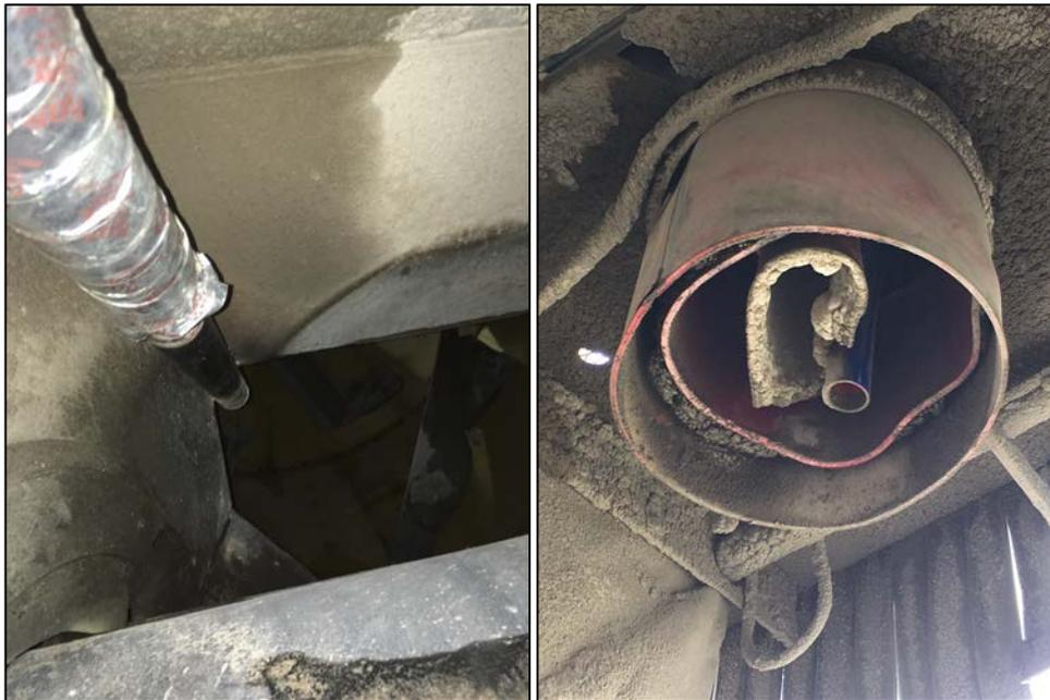
**Figure 3:** Location of injection nozzle in a central mixer application (left) and dry batch application (right).
