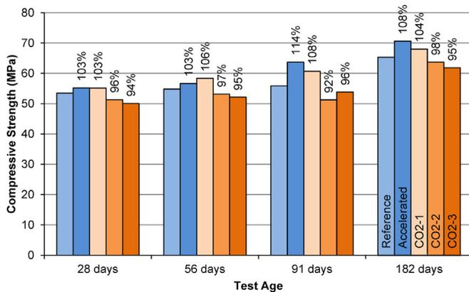
Fig. 3. Later age compressive strengths at 28, 56, 91 and 182 days.
