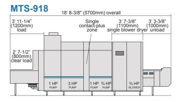
MEIKO's newest M-iQ fits small footprints while adding typical efficiencies of other M-iQs: heat recovery, blower dryer and high efficiency - available in steam or electric heat
