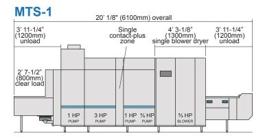
This M-iQ configuration works best for trayless cafeterias or kitchens with limited length available - ready to be installed with electric or steam heat
