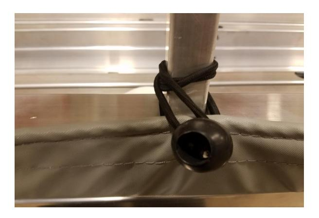
Older style canopy frame, (And end caps on new canopies). If your canopy has a lacer bar as shown, use this method to lace your cover. You can wrap the bungie cord around the lacer a few times to tighten it more.
