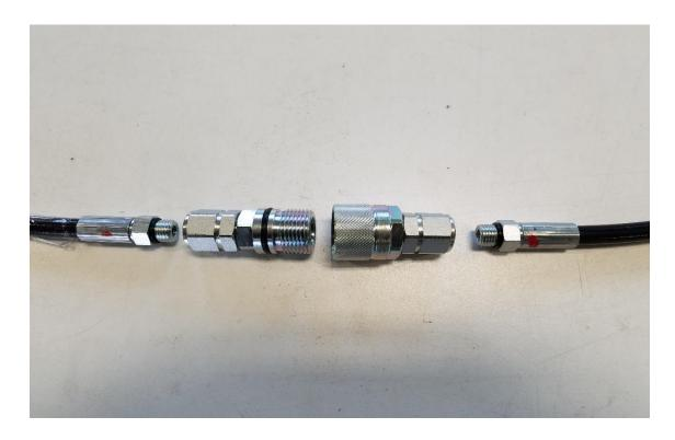
Disconnects here are separated from the hoses. Loosen one or both sides to release any back pressure that may have occurred when the pump was initiated. This will eliminate back pressure when tightening disconnects.
