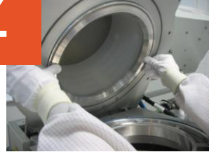
Deposition liner installation
