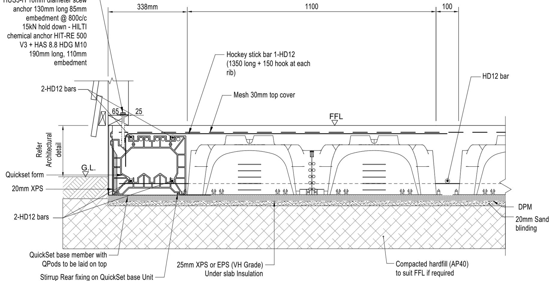
**QUICKSET TIMBER WEATHER BOARD QPod PERIMETER DETAIL**
