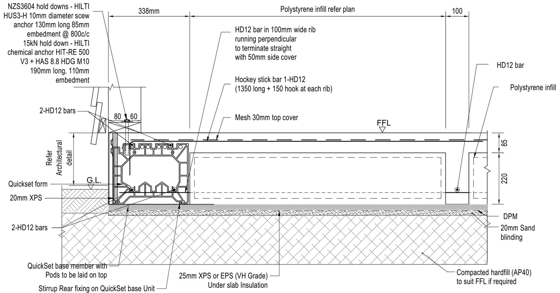
**QUICKSET TIMBER WEATHER BOARD PERIMETER DETAIL**
