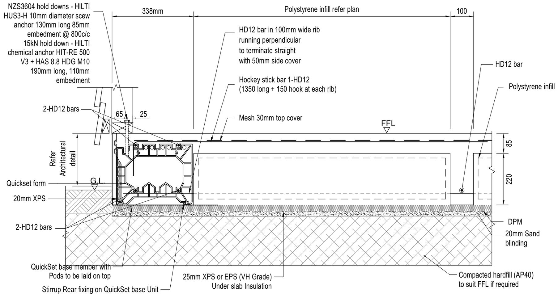
**QUICKSET TIMBER WEATHER BOARD PERIMETER DETAIL**
