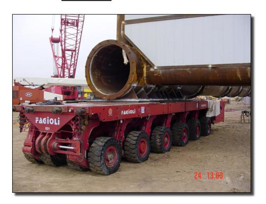
The support structures allowed for both longitudinal as well as lateral forces.
