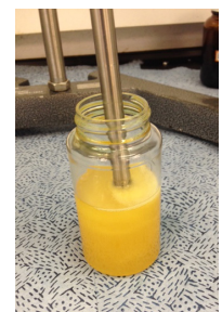
Figure 4. Homogenizing a sample of water-contaminated oil.
