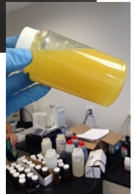
Figure 7. Sample which was shaken vigorously by hand for 30 seconds. To the eye, the opacity looks similar to the homogenized samples even though the water is not uniformly dispersed in the sample.
