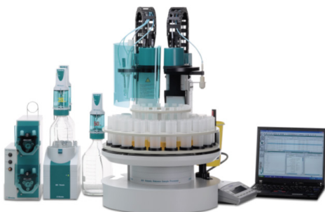
Metrohm Fully Automatic TAN and TBN Titration System
