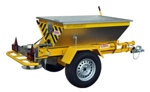
Logic's range of ground driven towed units are available in either 270L or 465L hopper capacity. The agitator, walking floor and spinning spreader disc are connected to a gear box and powered by the revolutions of the unit's axle this can be turned on and off so that the appliance is not spreading all the time.
