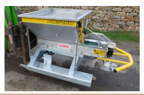
Mounted using fork tine pockets, this unit is secured with pins behind the tine uprights.
