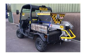
The de-mountable spreader is an ideal solution to any site which does not have access to tractors or telehandlers or is too small for a towed unit.
