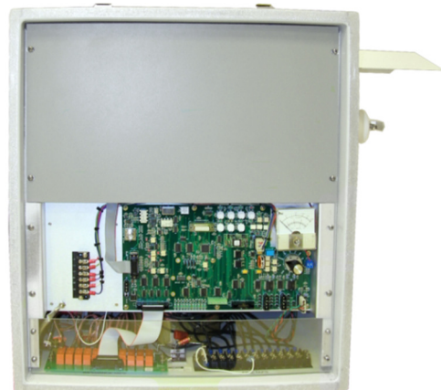
IP-66 Enclosure with Door Removed and Panels in Place
