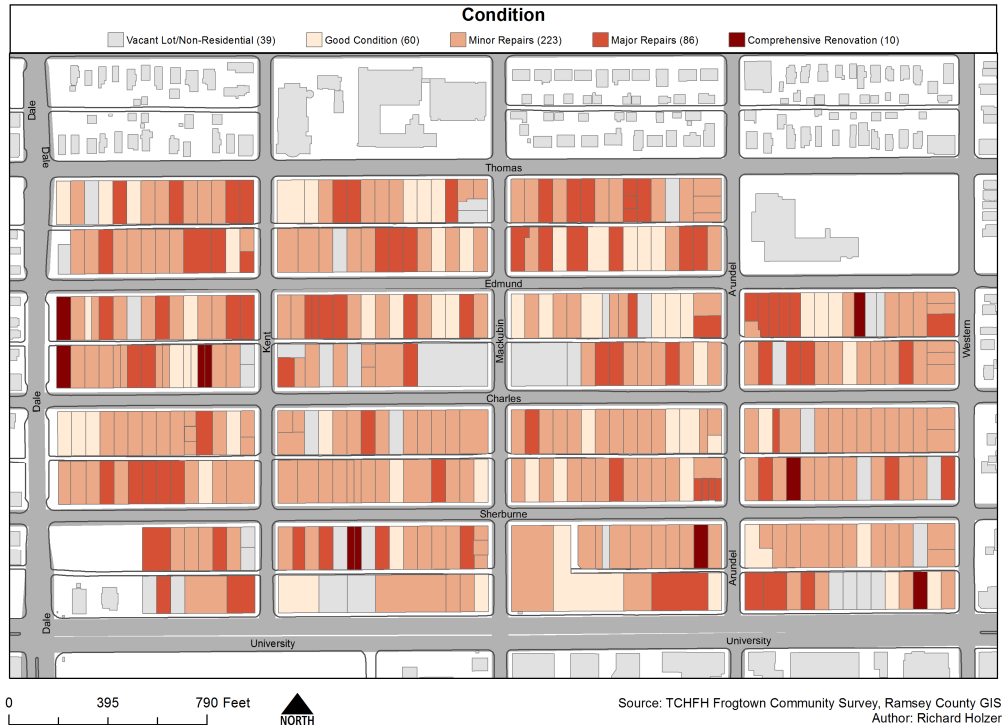
Figure 7 The overall condition of each building in the focus area,
