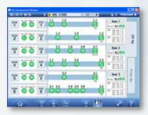
All valve, detector and chromatogram information is shown only for that specific SYS. Switching between the various SYS within the GC is as simple as touching the tab for that SYS on the HMI. Each SYS is assigned to specific GCMs for final data analysis and reporting.
