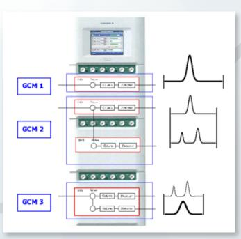
By dividing complex applications into smaller simultaneous measurements, the analyzer complexity as well as analysis time is greatly reduced.
